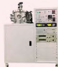
SE-300 - Magnetron sputter
