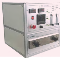
ETMS-1000 - Seebeck coefficient Measurement
