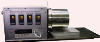
ETMS-1000 - Seebeck coefficient Measurement
