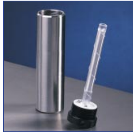
Electrolytic Hygrometer element and its stainless steel housing.
